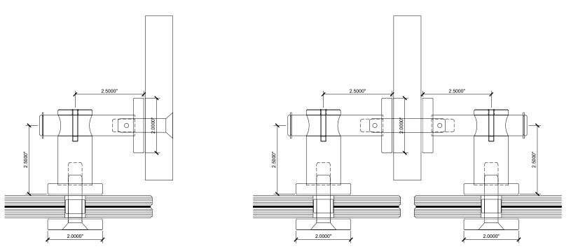
+ Manufactured with 316 stainless and specifically engineered to support heavy laminated glass with thickness between 9/16" and 11/16"
